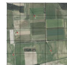
Figure 2. The method of the static cutting of the training images is shown. The black lines represent the cutting edges, the red dots the coordinates of the wind turbines.
